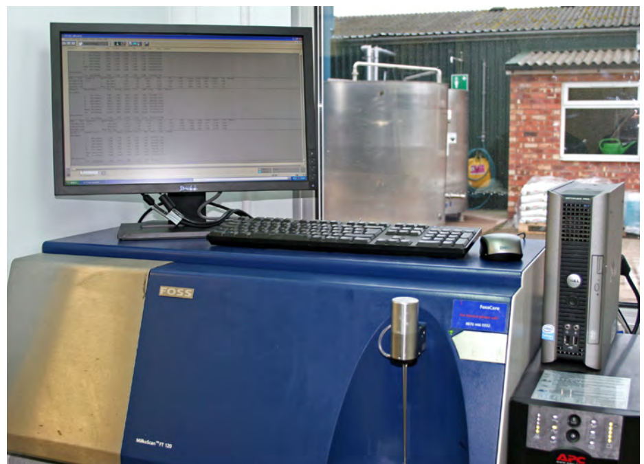
In addition to speeding up compositional testing, the MilkoScan™ offers a valuable new ability to test whey for protein content and permeate.
